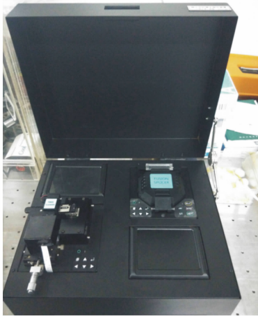
Fig. 6 All-in-one integration device for fiber welding and cutting
