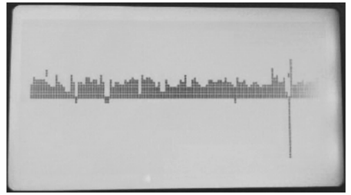
(a) 粗码位置发生误码的速度曲线图 (a) Diagram of velocity curve when fault code occurs in coarse code
